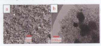
LiMnBO<sub>3</sub> particles are about 100 nm in diameter and are embedded in a porous carbon matrix. Electrochemical measurement results indicate that the LiMnBO<sub>3</sub>/C cathode exhibits excellent electrochemical performance.
