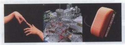
We evaluated the frictional force between two finger models that mimic properties of fingertips. Friction dynamics were drastically changed with the presence of fingerprints and variations in sliding speed and vertical force. For example, a periodic variation of the frictional force was observed under slow sliding conditions between finger models with fingerprint-like rough surfaces.
