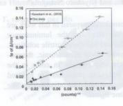
We improved Raman spectroscopic densimetry for a  $CO_2$  fluid using a micro-Raman spectrometer with high spectral resolution. The density precision of a new micro-Raman spectrometer is enhanced to  $\pm 0.0009 \, \mathrm{g \, cm^{-3}}$  by increasing counts, which is approximately one order of magnitude less than that reported in earlier studies.
