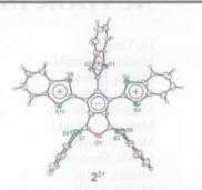
Spectroelectrochemistry of [5]radialenes with five 1,3-dithiol-2-yilidenes (DTs) (1) has been investigated. X-ray structure analysis of an oxygen adduct (2)2+(AsF6-)2(PhCI)1.5 reveals that 22+ has a structure of cyclopentadienide structure in the central five-membered ring.
